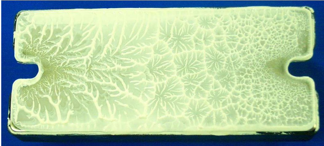
fig 4: SP4 base plate with properly applied thermal grease after removal from heat sink.
