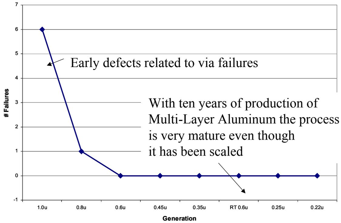
**Figure 1 : Failure Rate Versus Technology generations**
