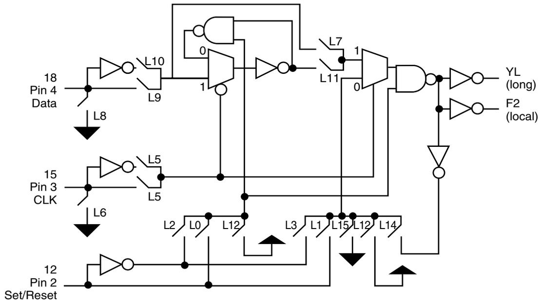
**Figure 2** • Architecture of the Logic Tile
