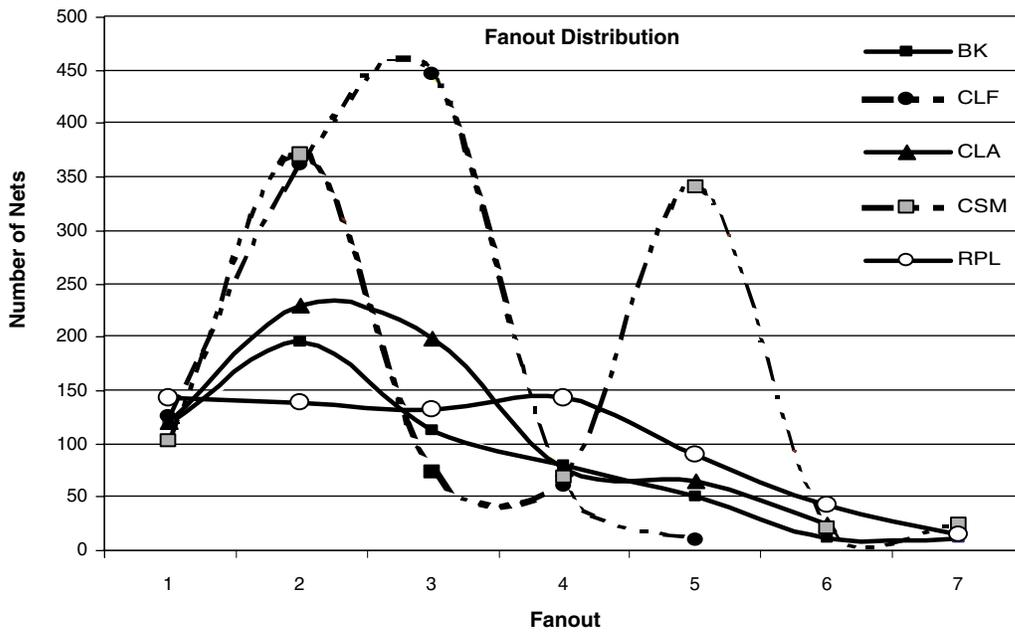
Figure 5 • Fanout Distribution for Various Adders' Internal Nets
