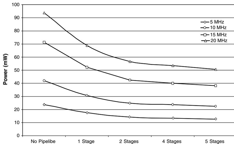
Figure 13 • ProASIC Power Characterization for 16-Bit Pipelined Multipliers
