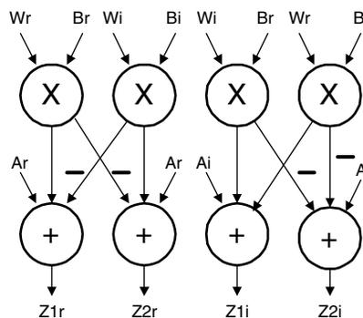
Figure 14 • Fast Fourier Transform (FFT) Block Diagram
