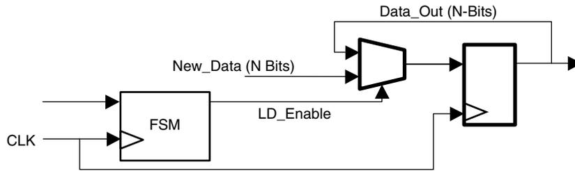
Figure 17 • Clock-enable N Bits Wide Register Implementation.
