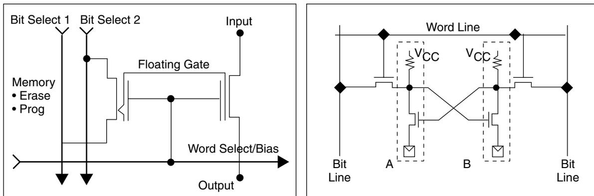
Figure 1 • Flash Switch vs. SRAM Switch
