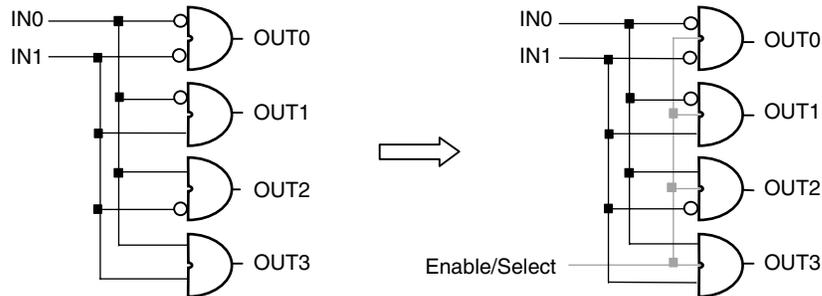
Figure 19 • Decoder with Enable
