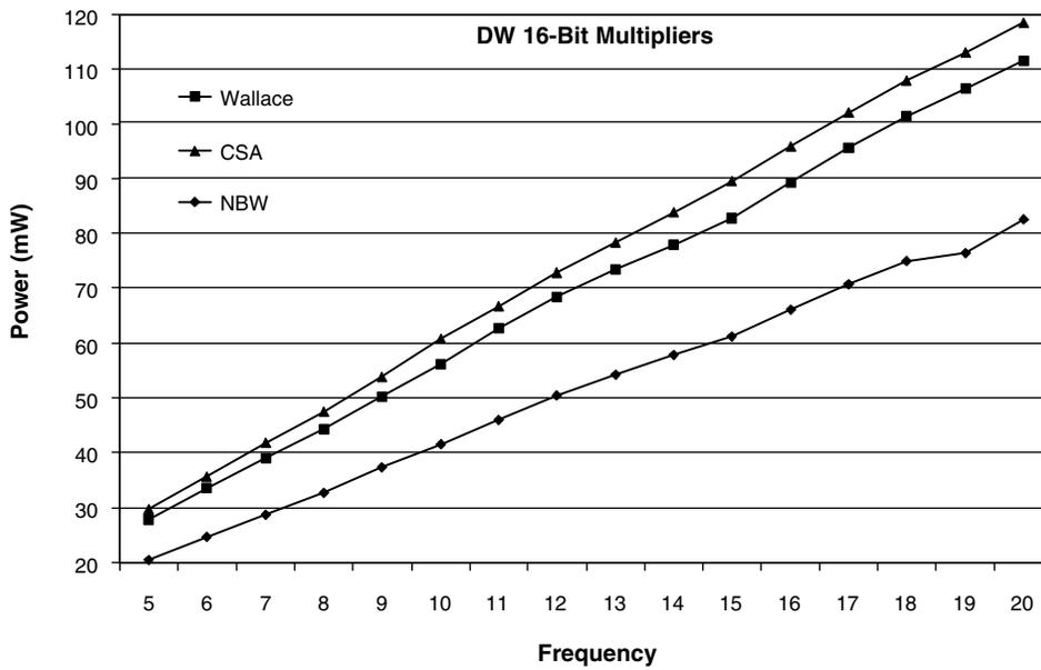
Figure 7 • ProASIC Power Characterization for various 16-bit Multipliers
