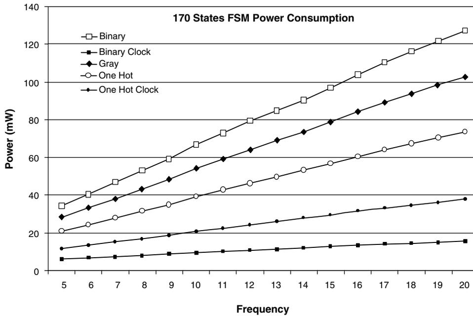
Figure 11 • Power Measure on ProASIC of 170 States Controller
